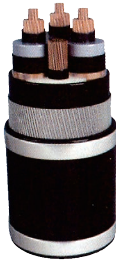
0.6/1kV, XLPE Insulated steel wire armored, PVC Sheathed Power Cable
